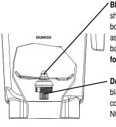
Blade Agitator Assembly. Use caution when handling the blade; it is sharp. When inserting the blade assembly through the container bottom, grip the blades with a soft cloth, align the flat sides of the blade assembly with the flat sides of the container. Place the retainer nut back on the inserted blade assembly and tighten clockwise. Do not force. Do not attempt to disassemble blade assembly.
